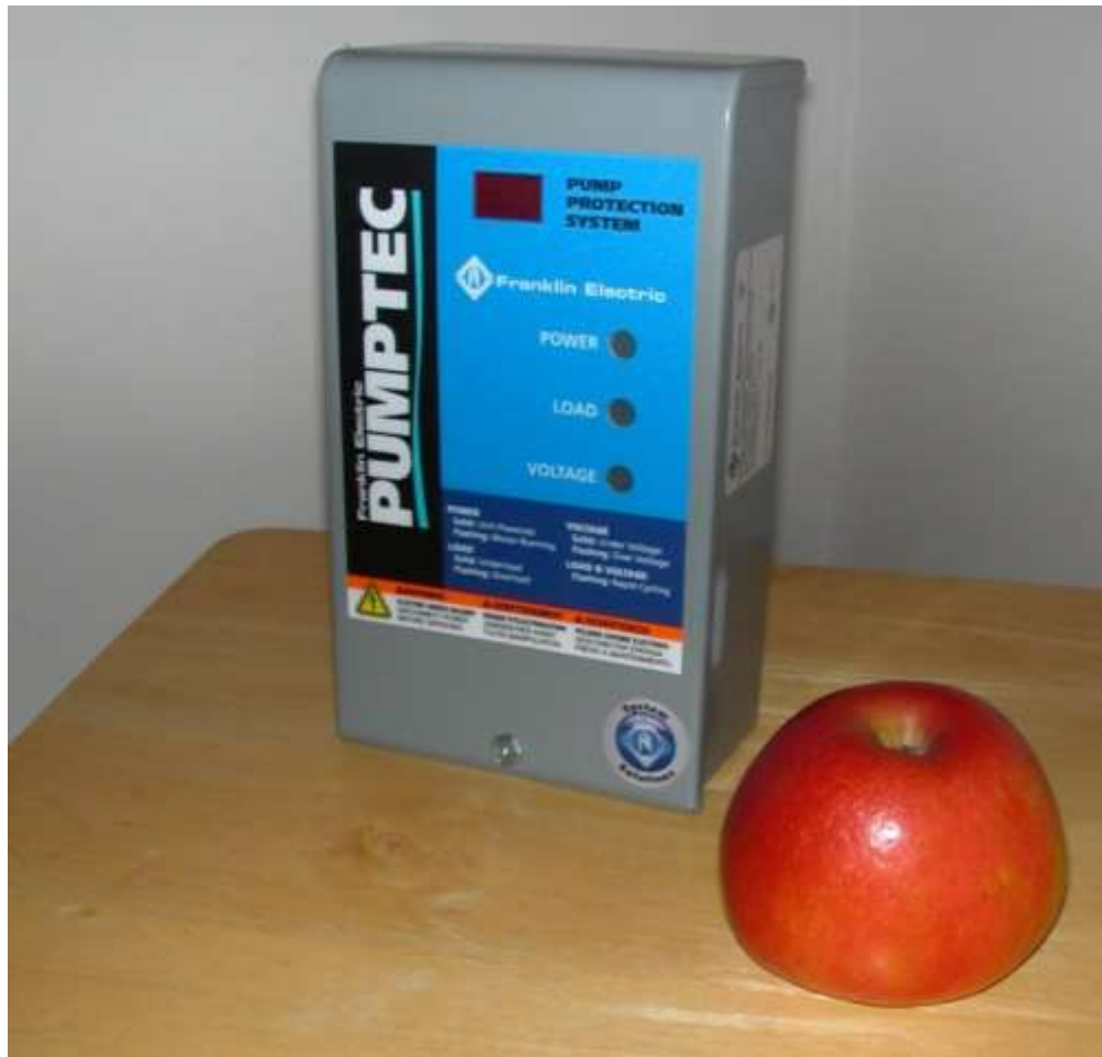
Pump Protection Box
